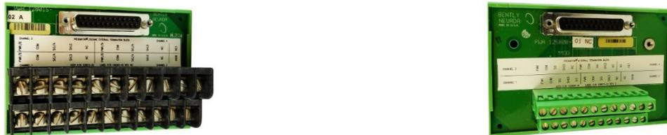
Figure 7: ET Blocks with screw terminals for lugged field wiring (left) and high-density "Euro" connectors for non-lugged field wiring (right)
